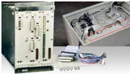
UPGRADE FOR POWER DRIVE With this power module it is possible to change a single circuit board. In case of a damage it is not longer necessary to change the whole unit.
