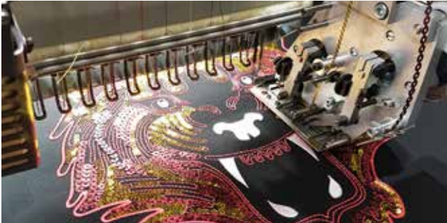
TWIN SEQUIN DEVICE T7 ( 2-9MM )
