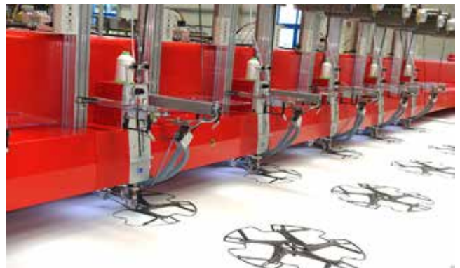
ZSK Technical System CZCW 0809- with eight W-Heads laying and fixing fibers.
